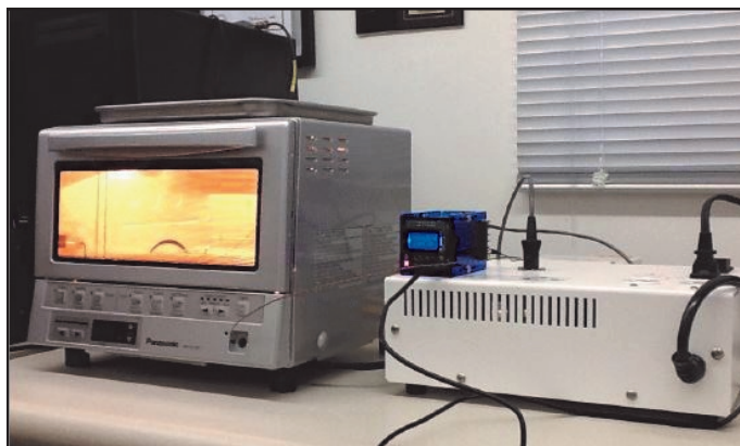
Illustration 6: Reflow oven in operation, with PID and SSR Cabinet
