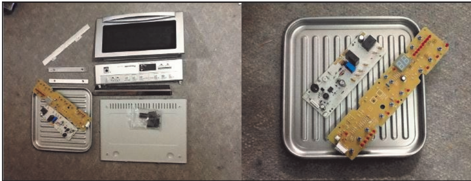
Illustration 3: Disassembled toaster oven (left) and "extra" boards (right)
